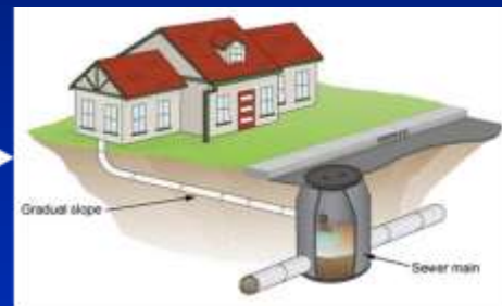
Conventional Gravity Sewer
